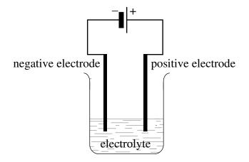
clear diagram containing all elements (power supply, connecting wires, electrodes, container and electrolyte);
